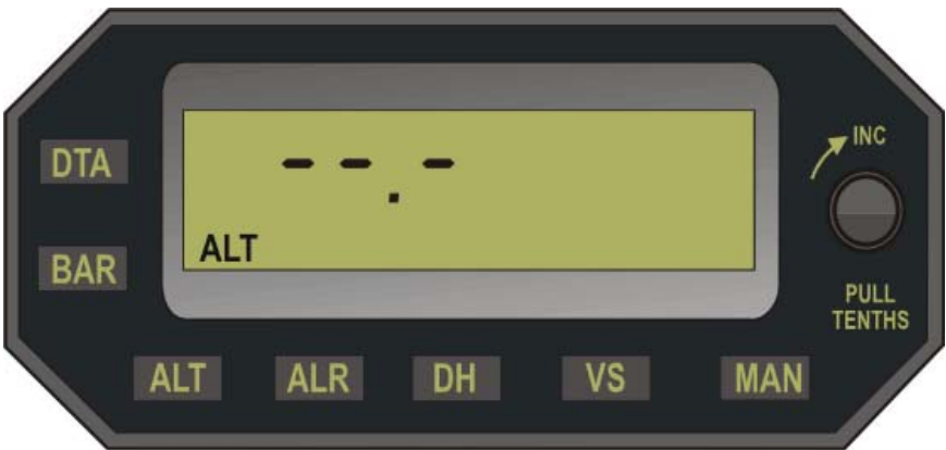
Fig. 3-1. Selector / Alerter Display, Loss of Encoded Altitude
